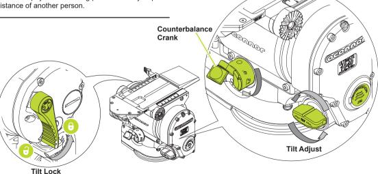
4. The payload C of G (Centre of Gravity) must align with the fluid head's tilt axis as shown below, slide the payload fore and aft using the camera plates sliding platform until the load is centered and balances upright in the vertical position with the tilt lock and drags off. Lock the tilt when done.
