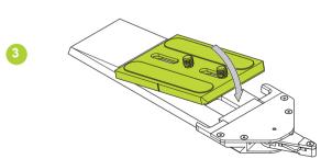
Replace the camera plate, the lever will snap in to the secure position.
