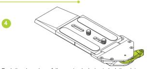
Push the clamp lever fully counterclockwise to lock the plate. Check the plate for movement and adjust again if necessary. The clamp lever should be operable with the pressure of just one finger.
