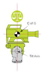
5. When the C of G of the camera is approximately over the tilt axis, adjust the counterbalance as follows. Hold the payload and release the tilt lock, then gently tilt the load from the horizontal position fore 30 - 45° and release slowly then aft 30 - 45° and release again, observing its response.
