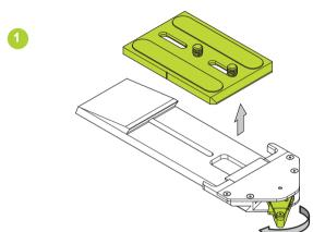
If movement is detected in the camera plate or the lock lever is to stiff, the clamp must be adjusted. Release the clamp lever (turn clockwise) and lift out the camera plate.
