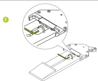
Using a hex key, adjust the small grub screw (clockwise to tighten the clamp and counterclockwise to loosen the clamp). Make small adjustments of between 1/8 and 1/4 turns.
